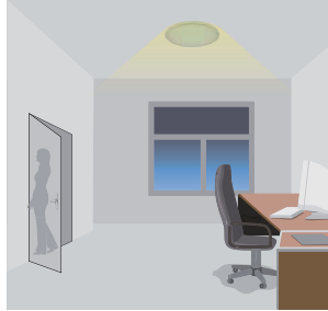
After hold-time, the light dims to stand-by level or turns off completely if surrounding natural light is above the daylight threshold
