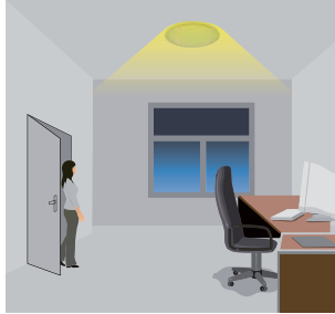
With insufficient natural light, the sensor switches the light on automatically when a person enters the room
